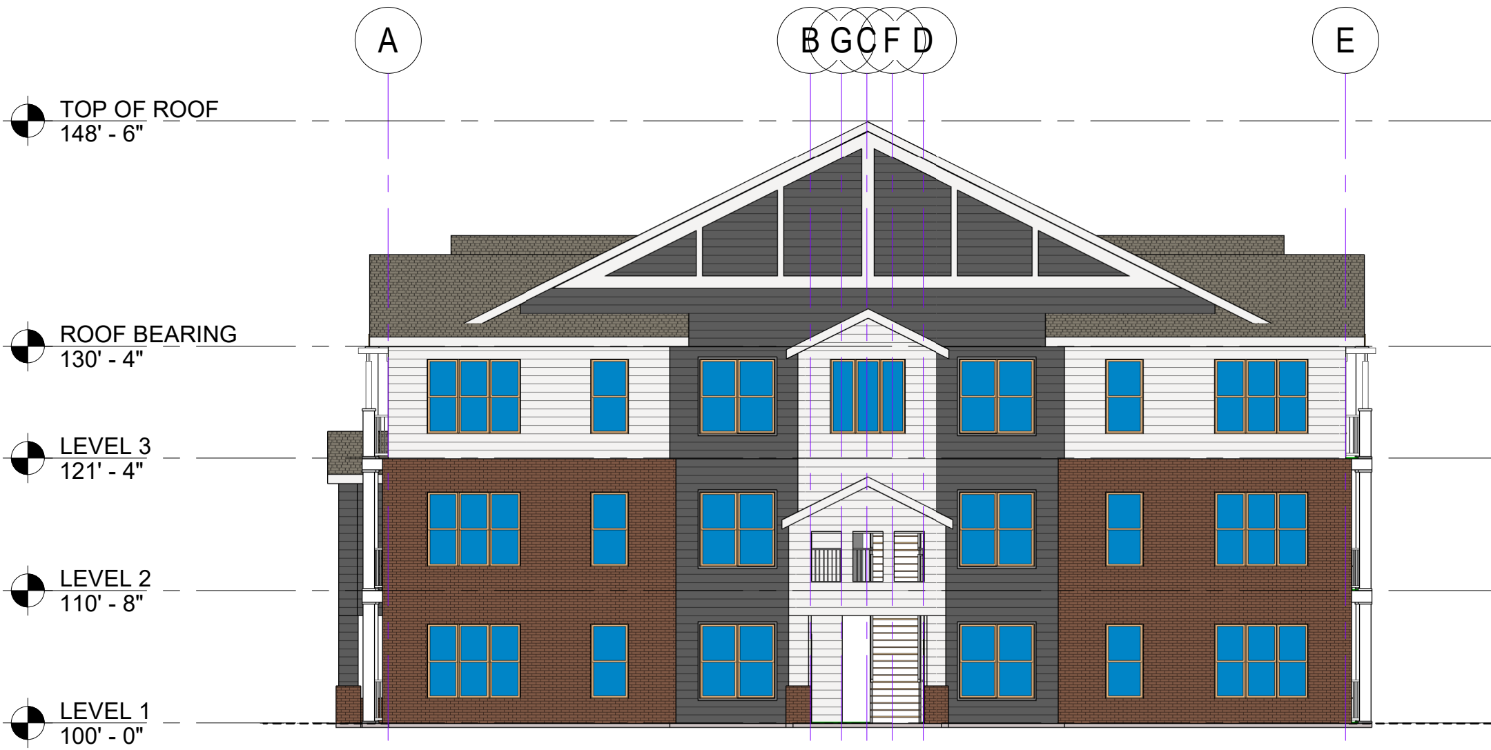
2 EXTERIOR ELEVATION - REAR A401-W1 3/32" = 1'-0"
